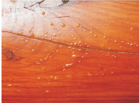
*Blisters in finish due to the presence of oil remaining in the wood.*
