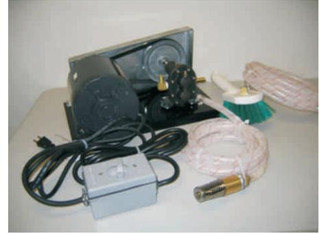
**Pump Designed to Apply Methylene Chloride**
