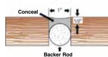
For joints 1" wide or more, the depth should be 3/8" to 1/2". The depth of joints less than 1" wide should be half the width but no less than 1/4". (Joint depth, overall, should be between 1/4" and 1/2".)
