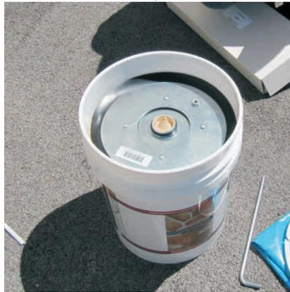
Place the follow plate on top of the product in the pail making sure that there is a good seal between the wall of the pail and the flexible edges of the follow plate.
