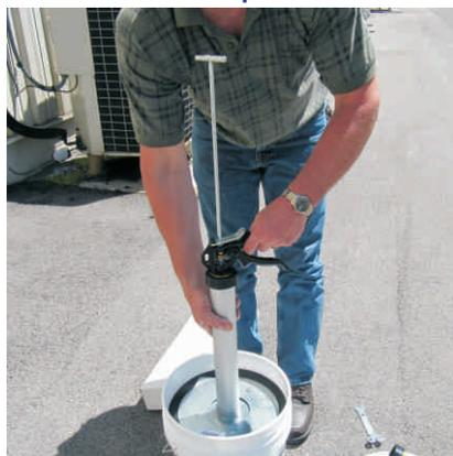
Once the rod is fully extended and the barrel is full of product, give the trigger one squeeze then disengage the barrel from the Follow Plate with a twisting motion.
