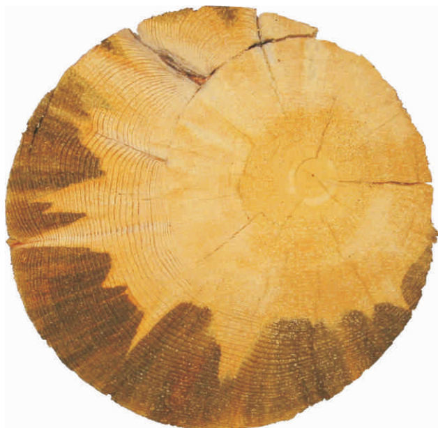
Cross section of blue stained log
