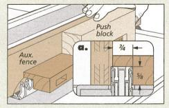
**Rabbet.** Set the dado blade to full width and install an auxiliary rip fence to cut the rabbet on the back outside edge of the stiles.
