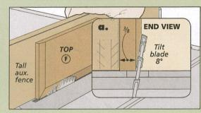
**Bevel the Top.** You can cut the 8° bevels on the top at the table saw by installing a tall auxiliary fence on the rip fence and tilting the blade.
