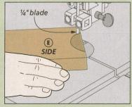
**Cut the Arc.** After marking the arc using a compass, go to the band saw to make the cut.
