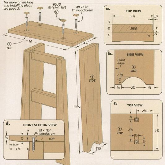
covered the screw holes with small squares of end grain oak.
