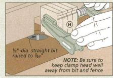
**Rout the Notches.** A clamp holds the blanks securely while you rout the notches using a straight bit.
