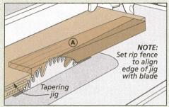
**Taper the Stiles.** With the stile fit firmly in the tapering jig, all you need to do is set the fence and make the cut.
