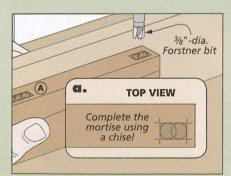
**Drill Mortises.** After laying out the size and location of each mortise, drill them out and square up the sides with a chisel.
