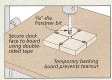
**Drilling the Clock Face.** After assembling the clock face, attach it to a backer board to drill the hole for the stem.
