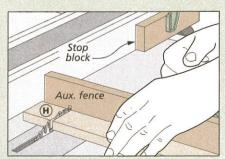
**Square Segments.** I attached a stop block to the rip fence to set the length for cutting the individual blanks.
