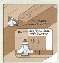
**Soften the Edges.** Round over the front outside edges of both stiles at the router table.
