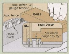
**Cut the Cheeks.** Bury part of the dado blade in an auxiliary rip fence and use a miter gauge to make the cheek cuts.
