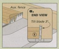
**Bevel Cuts.** Bevel the top and bottom edges of the sides using the miter gauge and auxiliary fence.
