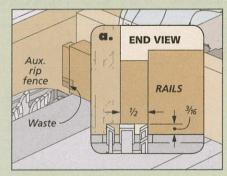
Then the Shoulders. You can use the same blade and fence setup to cut the shoulders of the tenons.
