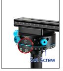
Point the lens to include the leftmost/rightmost region of interest. Loosen the set screw at the lower rotator index ring, rotate to align the **0**° mark to the reference mark. Tighten the set screw. Point the lens to include the rightmost/leftmost region of interest. Grab the **End** tab ring, rotate to align its black line to the reference mark.
