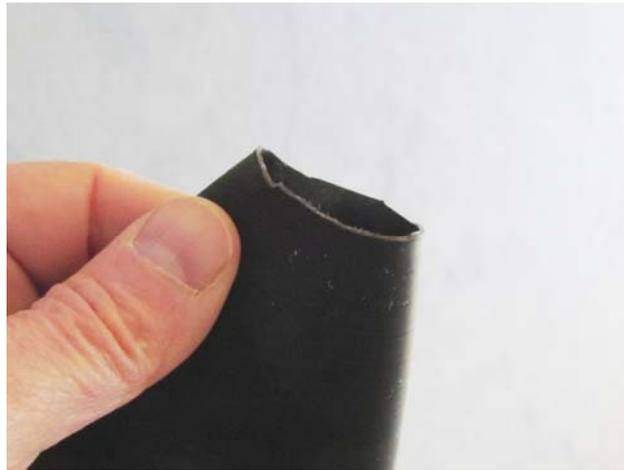
*A badly-trimmed wrist gasket. The notch could become a tear the first time you try it on, but it's not a lost cause. Work carefully to smooth out the rough edge.*
