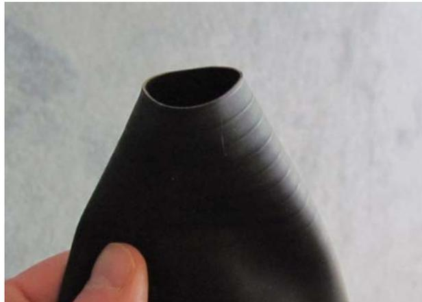
*A properly-trimmed wrist gasket has a nice smooth edge.*
