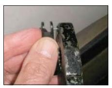
Push the roll pin into lever until 3mm exposed on the inner side.
