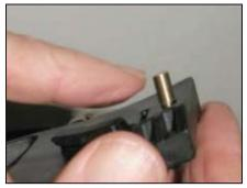
2. Assemble spring on locking pin shaft and insert locking pin in pedal with the chamber facing forward.
