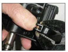
3. Hold the pedal in one hand with the locking pin pushed into the pedal. Slide lever/roll pin assembly over the end of the pin and insert the roll pin into the hole in the locking pin.
