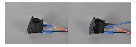
NOTE: The orange/white wire on the switch above is the power wire for the switch. The black wire is the ground for the light in the switch.
