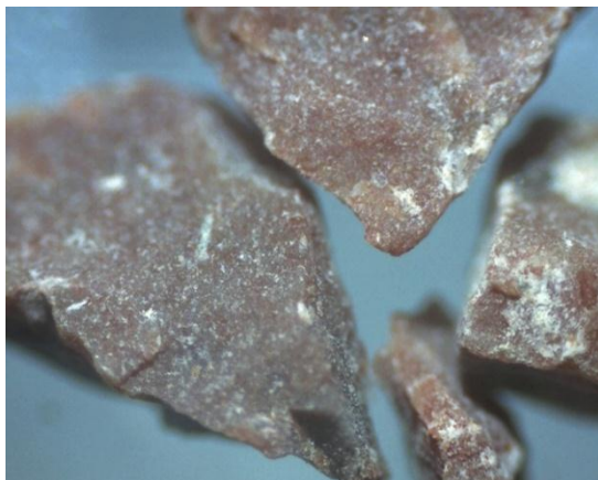
Figure 22: Microscope Images of Zeolite Media
