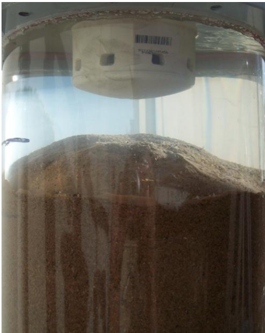
Figure 19: Photograph of the Compaction in the Sand Filter Bed
