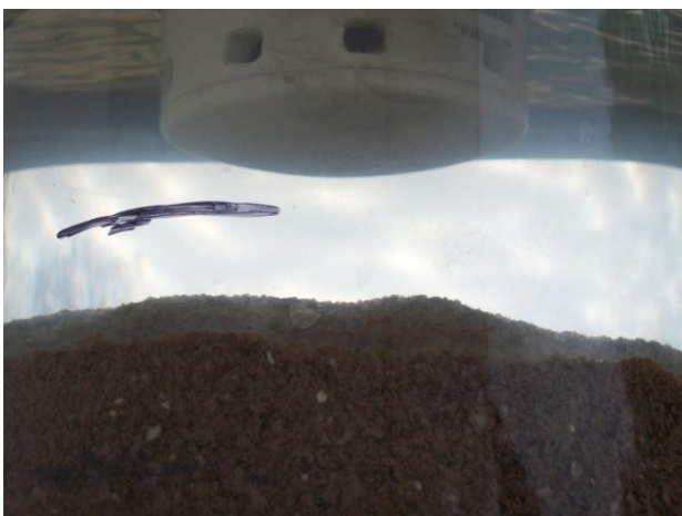
Figure 20: Photograph of the Compaction in the DiamondKleen™ Filter Bed
