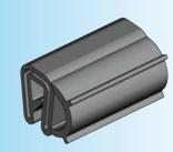
Hollow section (EPDM) black 45° ± 5 Shore A Clamping profile (EPDM) black 60° ± 5 Shore A
