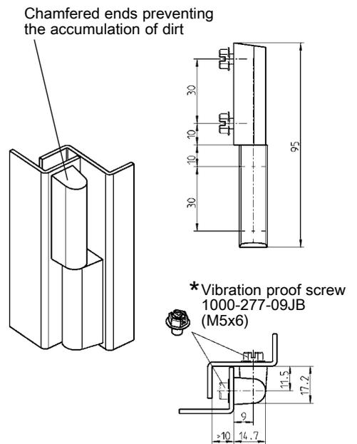
Plastic screw-on hinge polyamide GF black, pin stainl. steel and insert m.s. raw
