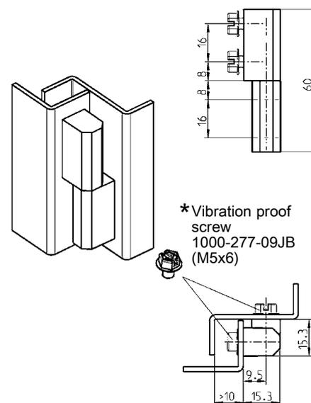
Plastic screw-on hinge polyamide GF black, pin stainl. steel and insert m.s. raw
