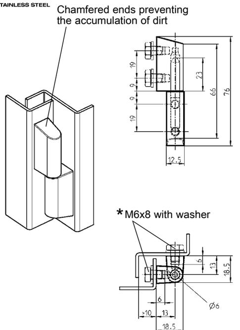
Stainless steel screw-on hinge AISI 316
