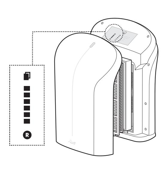
• Filter Maintenance & Replacement Light The Filter Maintenance and Replacement Light will illuminate when your air purifier needs attention.
