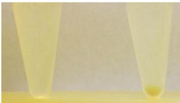
**Figure 4.** The colloids in a dilute solution (left) is concentrated into a small volume via centrifugation (right). Other strategies, including filtration, can be used to concentrate samples and remove impurities.
