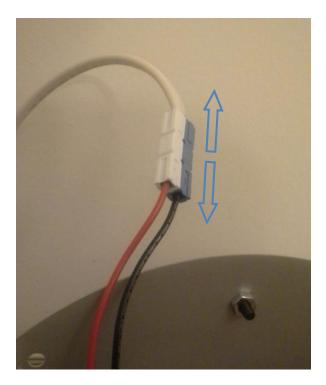
Step 2. Connect the purple-and-orange pair of click-connects from the remote control to the blue-and-white pair of quick connects in the LightPortal<sup>TM</sup>. Make sure to connect purple to blue and orange to white.
