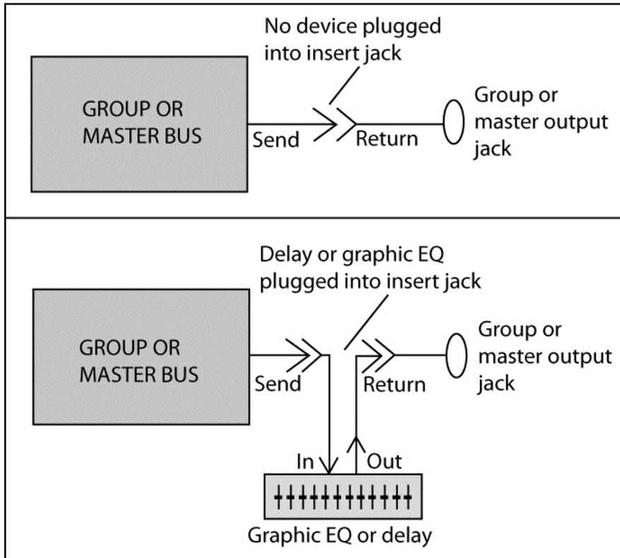
Figure 2. Plugging a device into an insert jack diverts the signal to and from the device.
