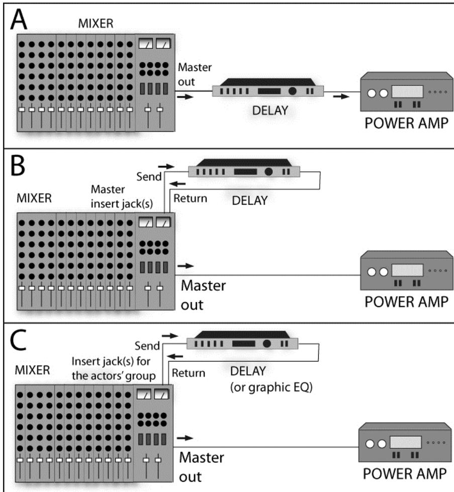
Figure 3. Three ways to connect a delay unit to a sound system.
