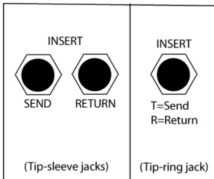
Figure 1. Two types of insert jacks.
