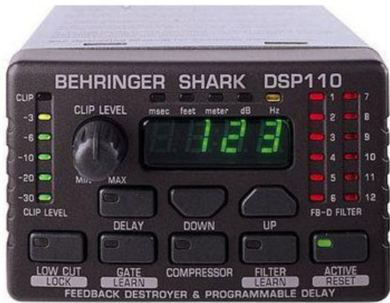
Figure 3. An example of an audio delay unit.
