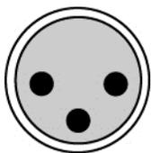
*A female XLR connector has three holes. A MIC IN connector looks like this.*
