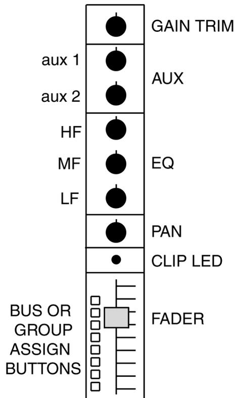
Suppose you want to control the volume of certain types of mics all at once with a single bus fader. For example, you might send all the floor mics to Bus 1, all
