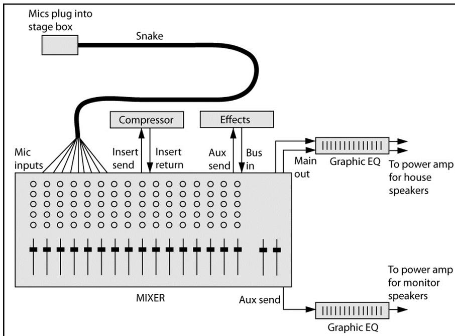
Mixer connections. Insert send and Insert return are not covered in this article.
