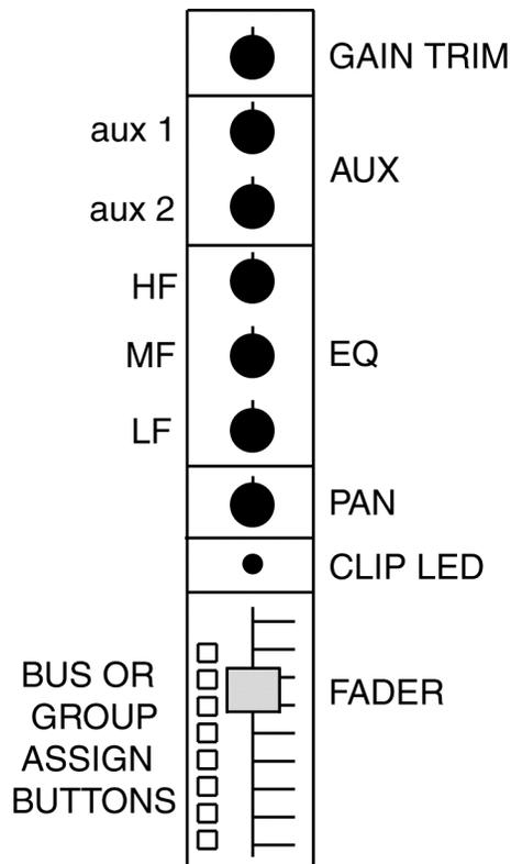
*A channel strip has all the controls for one microphone's signal.*
