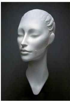
Fig. 6. Example of a headworn mic, the Countryman E6i Omni EarSet.
