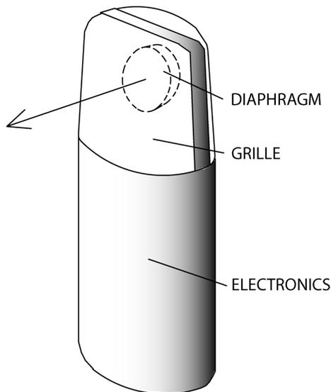
*Fig. 6. A typical multi-pattern mic that is side-addressed.*
