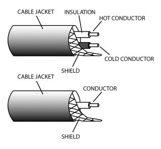
In a balanced cable, the signal in one wire is in opposite polarity with the signal in the other wire. When the signal voltage goes positive in one wire, it goes negative in the other wire.
