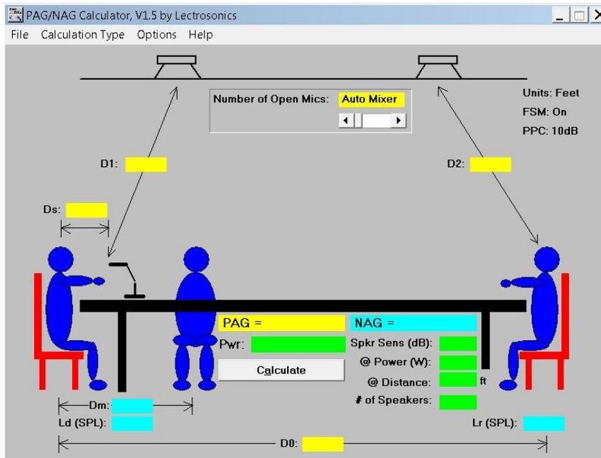
First, under “Calculation Type” at the top, select “single speaker”. Under “Options” uncheck “calculation warnings”. Set the “Number of Open Mics” to 1. Set  $D_m$  to 20, set  $L_d$  to 70, and set  $L_r$  to 70.
