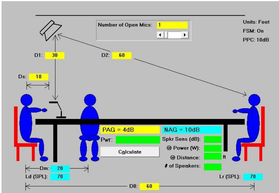
The Needed Acoustic Gain to make speech heard adequately is 10 dB, but the system can provide a Potential Acoustic Gain of only 4 dB. It won't be loud at all. If you turn up the mic loud enough to hear the speech, the system will feed back. That's why I don't recommend using a loudspeaker over the stage. It's too close to the mic and too far from the audience.
