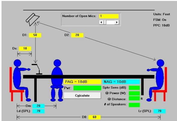
Here's a handy calculator that predicts how loud a sound system can get without running into feedback. You enter various distances related to the mic and speaker placement, and the calculator tells you how likely the system is to go into feedback.
