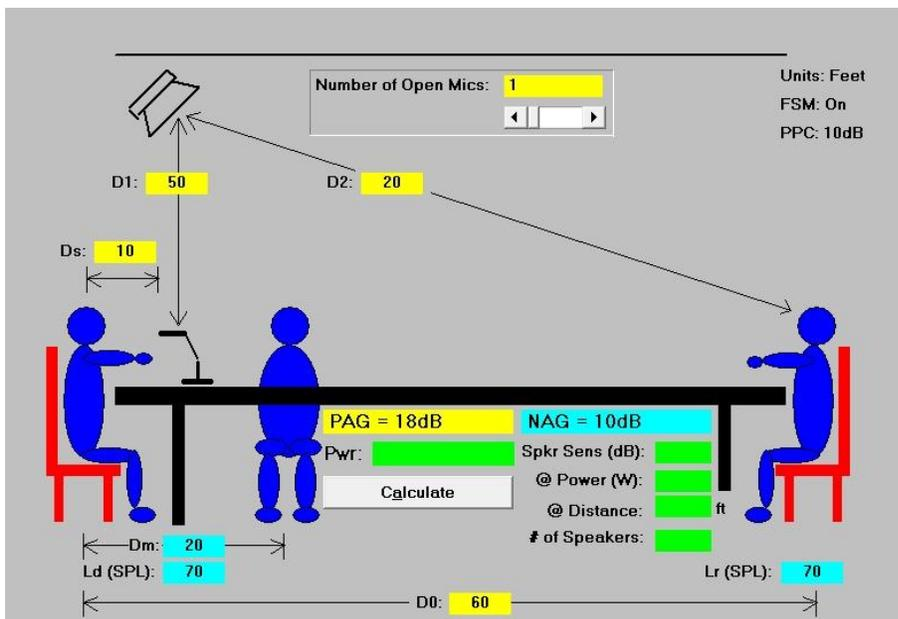
Under “Options” at the top is a selection called FSM or Feedback Stability Margin. To prevent the sound system from ringing, you want to operate it at 6 dB or more below the Potential Acoustic Gain. In other words, turn down the sound system 6 dB below the point of ringing. If the FSM option is checked, the calculation includes the Feedback Stability Margin, which is good practice.
