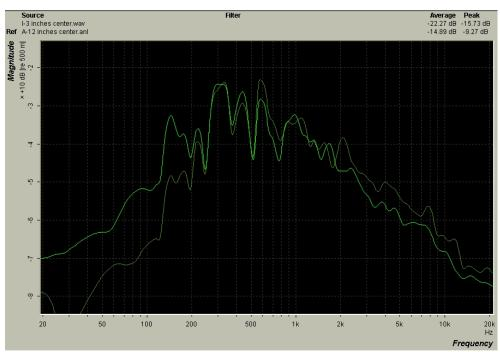
Red curve: Spectrum measured 1 foot from the center of the banjo. Yellow curve: Spectrum measured 3 inches from the the center of the banjo.
