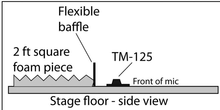
*TM-125 floor mic in an L-shaped cardboard baffle, with a foam piece behind to block sound from the pit orchestra (the TM-125 is now the Stage Floor Mic)*
