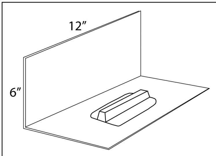
*TM-125 floor mic in an L-shaped cardboard baffle*
