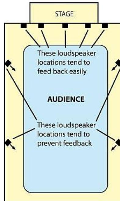
Fig. 5. Speaker placement vs. feedback.
