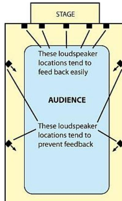
Fig. 5. Speaker placement vs. feedback.
