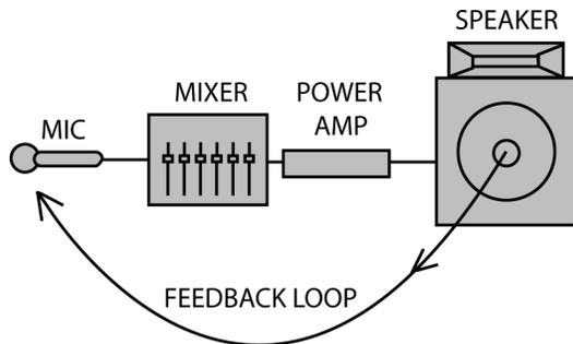
Fig. 1. The components in a feedback loop.
