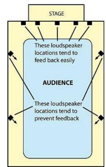
Fig. 5. Speaker placement vs. feedback.
