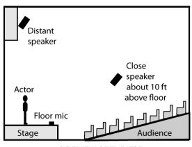
SIDE VIEW OF THEATRE Fig. 4. Distant and close speaker placements. Close placement has less feedback.
