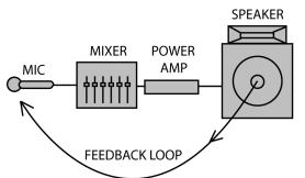
Fig. 1. The components in a feedback loop.
