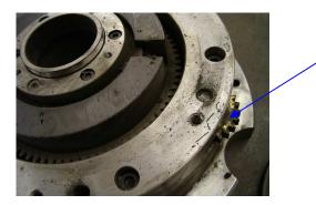
Worn transfer gear due to poor clearance during alignment. Place lower set in position with fixing screws loose & then moved forward to allow slight clearance between two brass gears. Securing screws should then be tightened.
