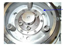
Upper set is heavily contaminated with nickel dust. Ensure stamper is clean thus preventing premature wear on cutting parts.
