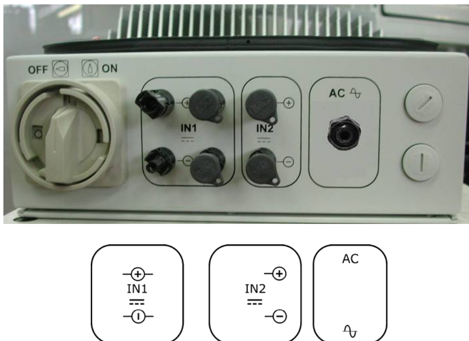
Fig. 10. Connectors found on inverter bottom and their labels (PVI-4.2)
