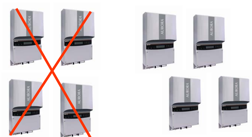
Fig.7 Recommended installation of AURORA inverters
