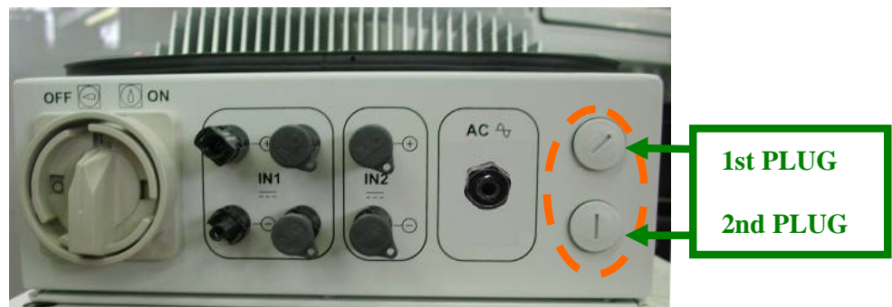
Fig.23 Holes for cables necessary for RS-485 port connection or wiring for RJ12 connectors connection.
