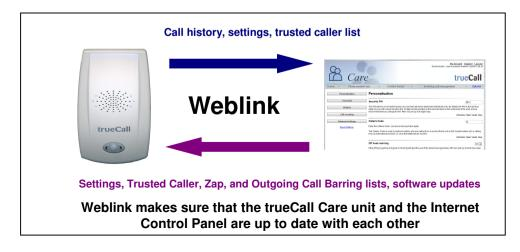
You can perform a manual Weblink at any time by pressing down trueCall's button and holding it down for two seconds. Wait for it to 'beep' then release the button.
