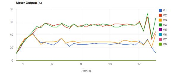
In this case, you can see the odd motors is outputting less power than even ones. The odd ones M1 and M3 is taking effect on right rotation (yaw to right), they use less power to keep the heading when hovering. It means the copter might have this reaction: to your yaw control, the copter turns to right very easy; but when yaw to left, the copter seems labored. **Solution:** check the motor installation; reinstall the arms or motor mounts if needed.
