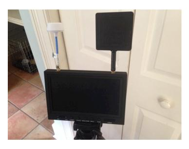
Setting up the video monitor is pretty simple, just screw the monitor to the tripod (the hood is optional and recommended in sunny conditions) and attach the round antenna to the left side and square patch antenna to the right side. The mushroom antenna is unidirectional and can pick up signals in all directions. Think of it as a light bulb emitting a small amount of light in all directions. The square antenna is called a patch
