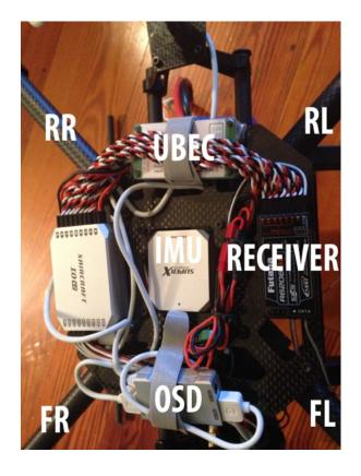
The OSD takes info from the IMU and overlays it onto the video input into the module. That video is then output to the video transmitter.
