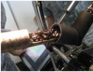
oil and sometimes carbon are built up on the inside of the drum. This process of seasoning will imbed the pores of the metal with oil.
