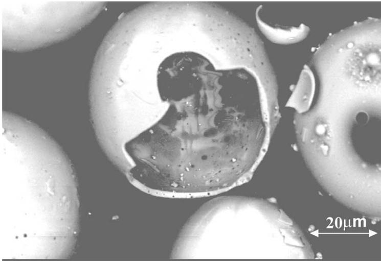
Fig. 2. SEM micrograph of broken cenosphere showing its hollow characteristics and porous walls.
