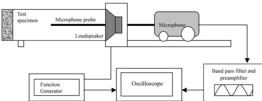
Fig. 3. Schematic of experimental setup used for acoustic characterization.
