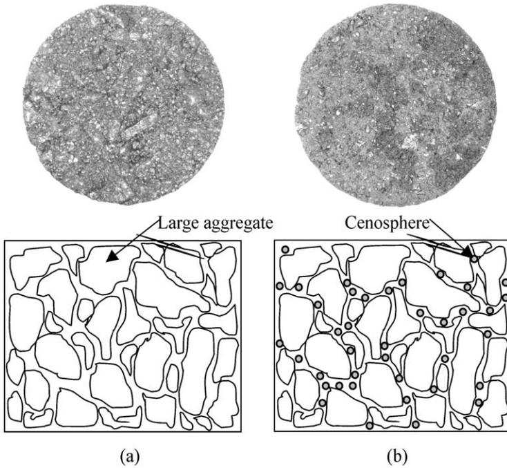
Fig. 11. (a) Structure of asphalt specimens without cenospheres (b) Structure of cenosphere-rich asphalt specimens.
