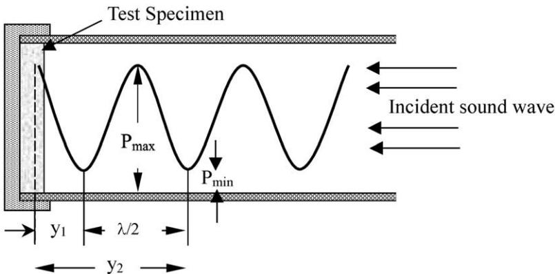
Fig. 1. Cross-section of impedance tube showing variation of pressure as a function of distance from the specimen.
