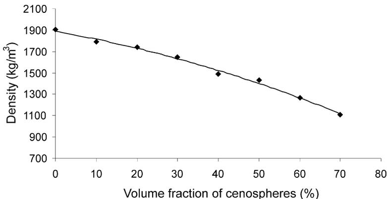
Fig. 4. Mass density of cenosphere-rich cement concrete specimens as a function of volume fraction of cenospheres.
