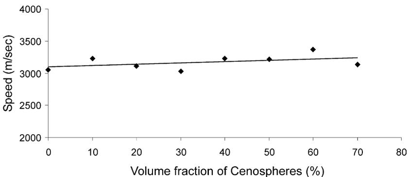
Fig. 6. Dilatational wave speed as a function of volume fraction of cenospheres in cenosphere-rich cement specimens.
