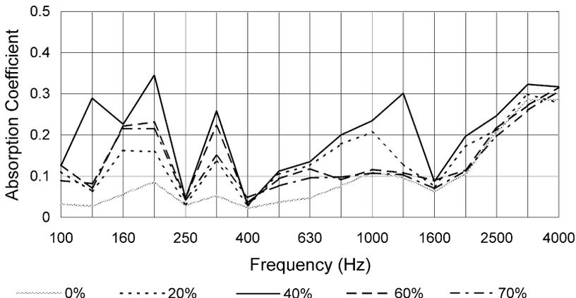
Fig. 7. Absorption coefficient as a function of volume fraction of cenospheres for 25 mm thick cenosphere-rich cement specimen.
