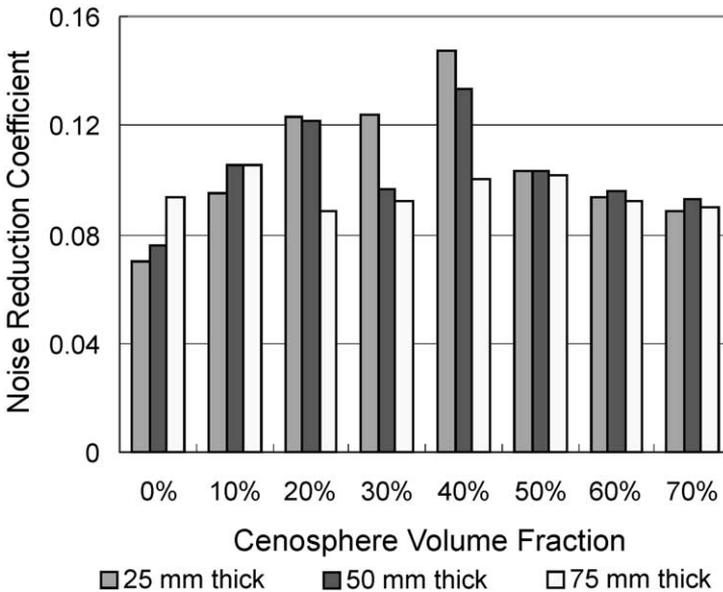
Fig. 9. Noise reduction coefficient as a function of cenosphere content for different thickness of cenosphere-rich cement.
