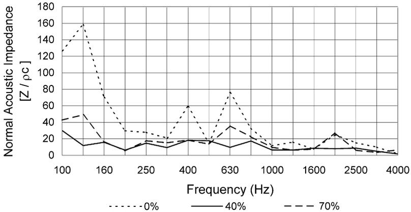
Fig. 8. Normal acoustic impedance as a function of frequency for 25 mm thick cenosphere-rich cement specimen at different cenosphere volume fractions.
