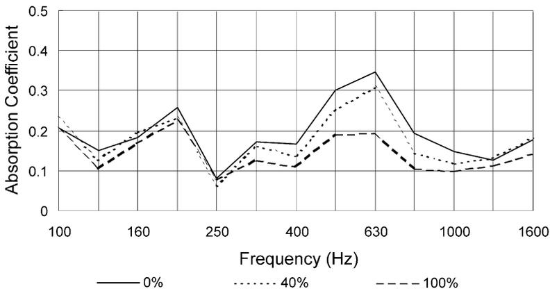
Fig. 10. Absorption coefficient as a function of frequency for 64 mm thick cenosphere-rich asphalt concrete specimen at different cenosphere volume fractions.
