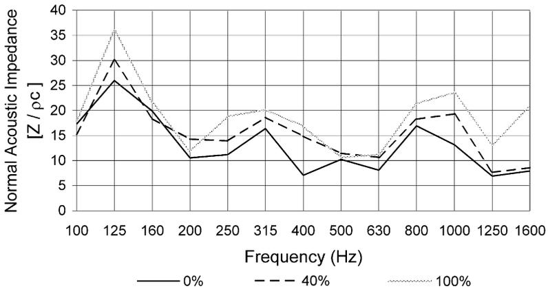
Fig. 12. Normal acoustic impedance as a function of frequency for 25 mm thick cenosphere-rich asphalt concrete specimen at different cenosphere volume fractions.
