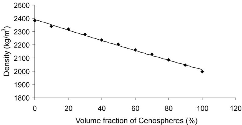
Fig. 5. Mass density of cenosphere-rich asphalt concrete specimens as a function of volume fraction of cenospheres.
