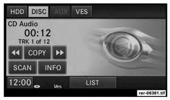
2. Touch the COPY soft-key to copy music tracks of the inserted disc to the Hard Disk Drive.
