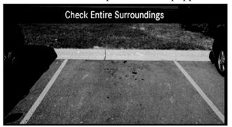
When equipped with Parkview®, the radio display shows the rear view camera picture as soon as the shift lever is in the R position for vehicles with automatic transmission. In vehicles with manual transmission the reverse gear must be engaged.
