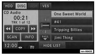
Toggle between the media and the radio menus by pressing the RADIO/MEDIA hard-key. The different media modes can be selected via the tabs in the radio screen.
