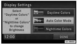
Select the Daytime Colors soft-key to switch to manual daytime mode and to adjust the brightness of the display using daytime colors.
