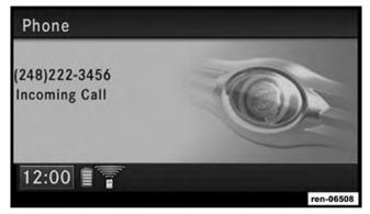
Uconnect<sup>TM</sup> Phone is fully integrated with the vehicle's audio system. The radio display will be used for visual prompts from the Uconnect<sup>TM</sup> Phone system such as phone battery status, signal strength, caller ID, and call type.
