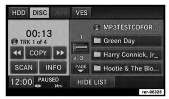
A MP3/WMA disc may contain audio files in a folder structure. The folder, if any, is shown in the list view.
