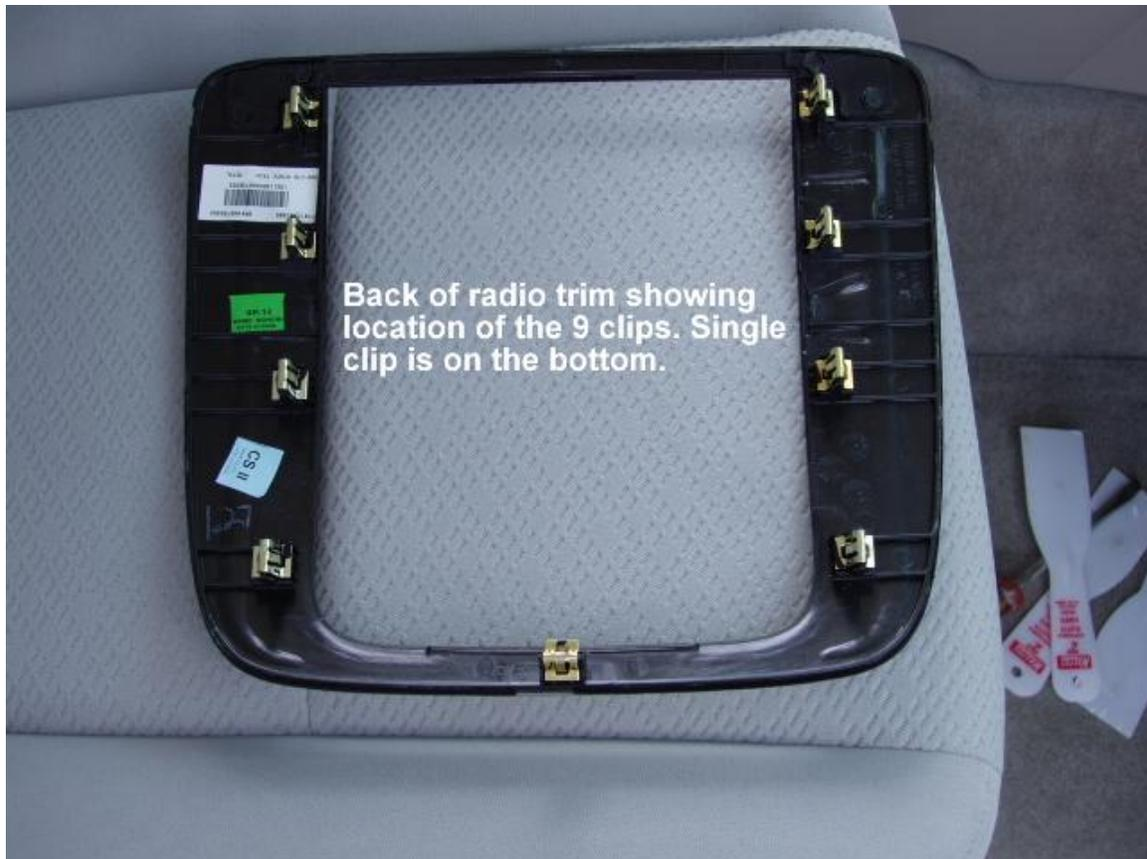
**Using a plastic trim removal tool or 2 plastic putty knives along with a screwdriver, remove the radio trim bezel. Note: there are no screws to remove and be careful not to scratch your bezel.**
