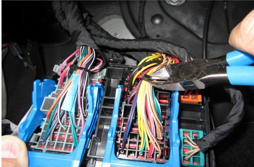
**Carefully cut the wire-tie to see the wires more easily. Locate a green with a white striped wire.**
