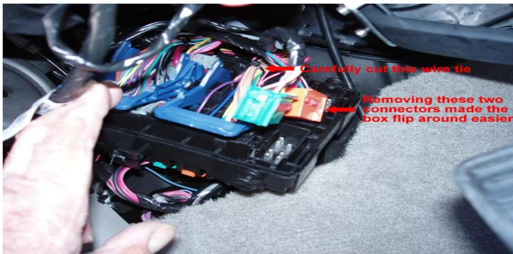
Remove the 2 connectors as shown in the picture to easily flip the box around.
