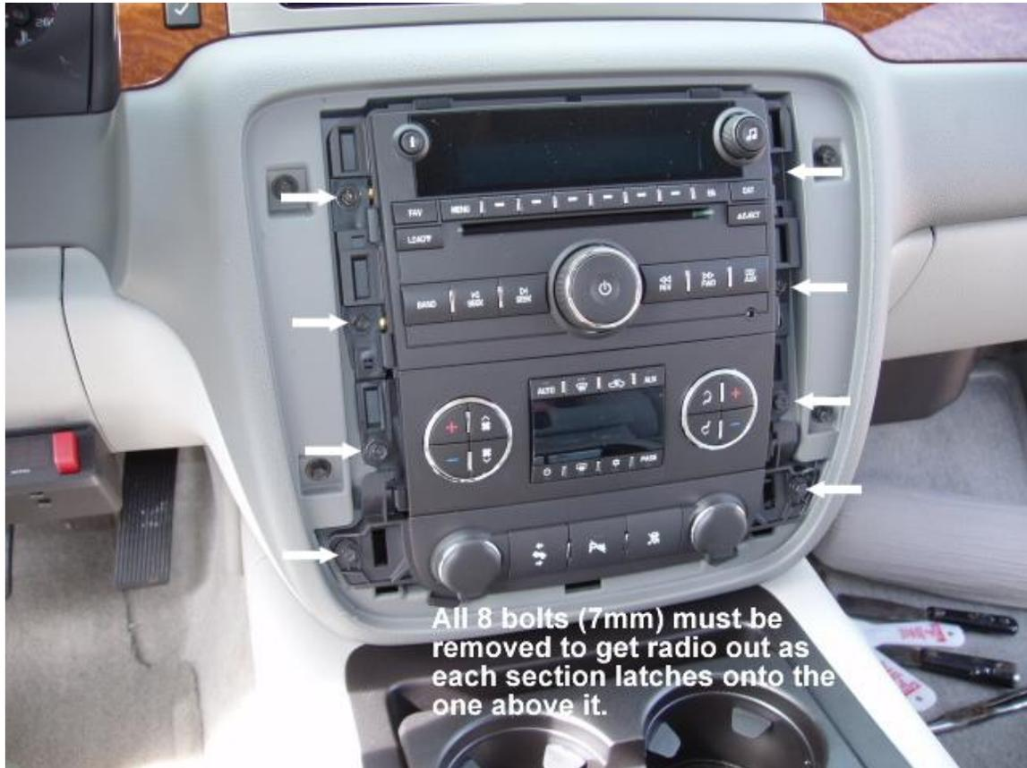
**Remove all 8 (7mm) bolts to remove radio, a/c controls and lighter panel. Now slide radio out, disconnect all radio connectors (not the AC or lighter panel connectors) and the FM antenna.**
