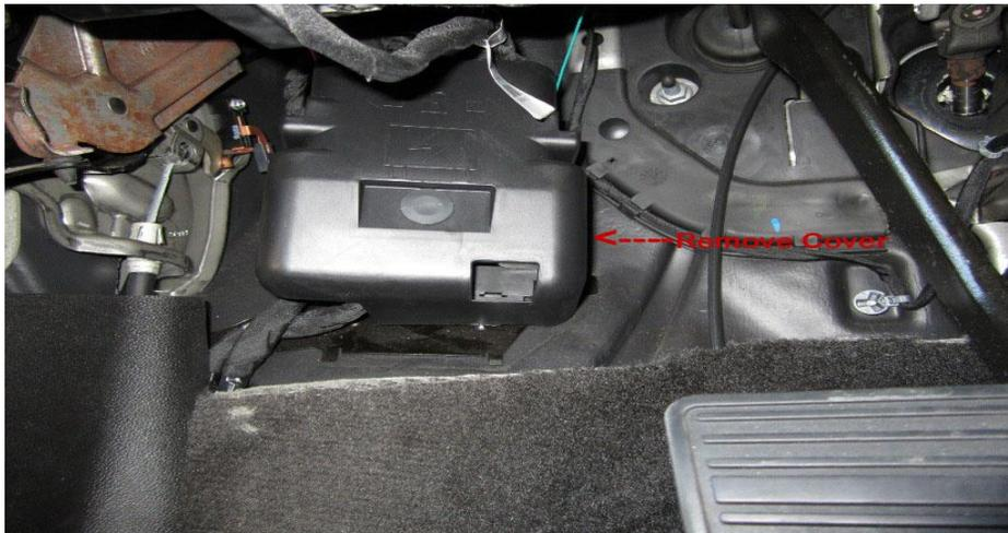
Locate the wiring box under the dash to the left of the brake pedal. Remove the cover. After the cover is removed, flip the box over to expose the wires on the back of the box.
