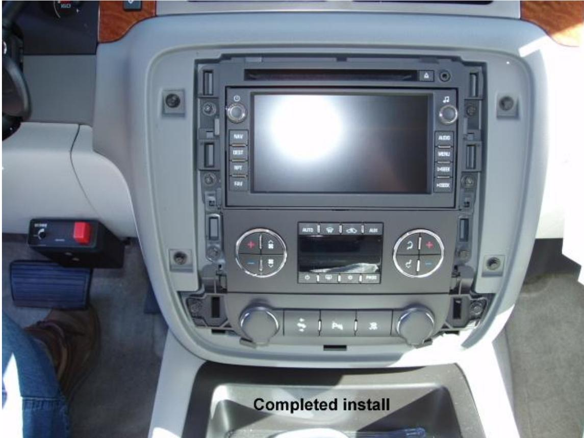
**Slide the navigation unit in along with the AC controls & lighter panel.
