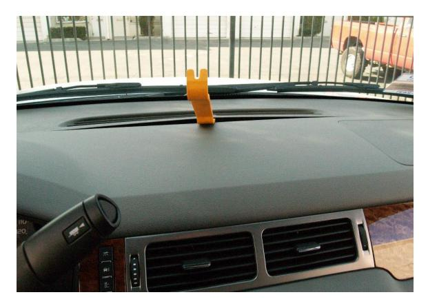
Using a plastic trim tool or a screwdriver, pry up the top dash panel as much as possible to install the GPS antenna module.
