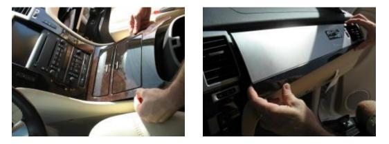
2. NEXT, THE PANEL SURROUNDING THE SCREEN AND RADIO IS POPPED FREE FROM ITS FRICTION CLIPS AND THE 2 CONNECTORS ON THE BACK OF THE TRIM IS UNPLUGGED TO ALLOW IT TO BE FULLY REMOVED. THIS WILL EXPOSE THE 7MM SCREWS HOLDING THE SCREEN/RADIO ASSEMBLY IN PLACE.
