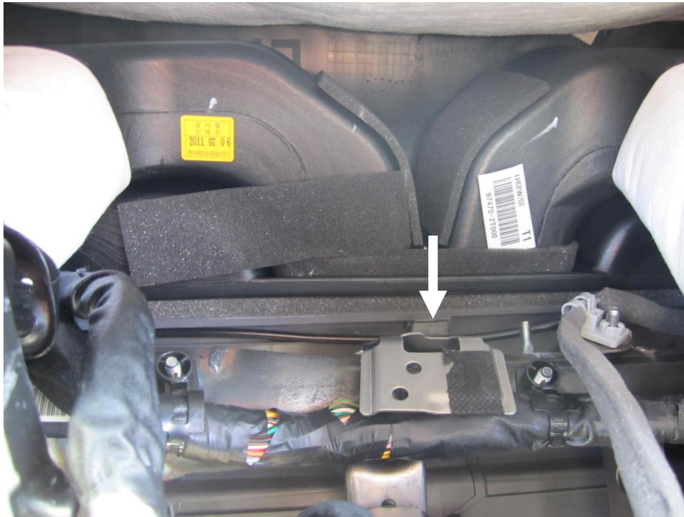
Bend the audio support bracket downwards.
