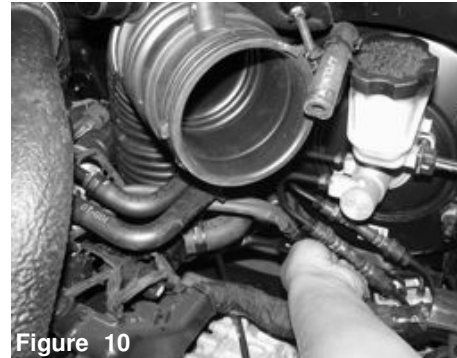
Figure 10 From the bottom side of the intake air duct, loosen the clamp with a 10mm socket/ratchet attached to the turbo inlet.
