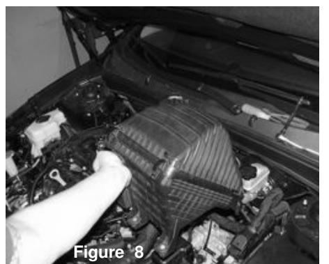
Figure 8 You may now pull the entire air box assembly out of the engine bay by lifting up and out.
