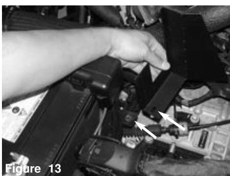
Figure 13 Behind the battery, Align the hole on the Injen air diverter with the pre-threaded hole where the left bolt that once attached the factory air box assembly too.
