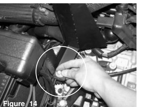
Figure 14 Place a M6x16 bolt and a fender washer onto the air diverter and attach it to the threaded hole.
