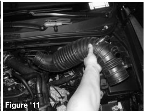
Figure 11 Detach the intake air duct from the turbocharger and you may now remove the intake air duct from the engine bay.
