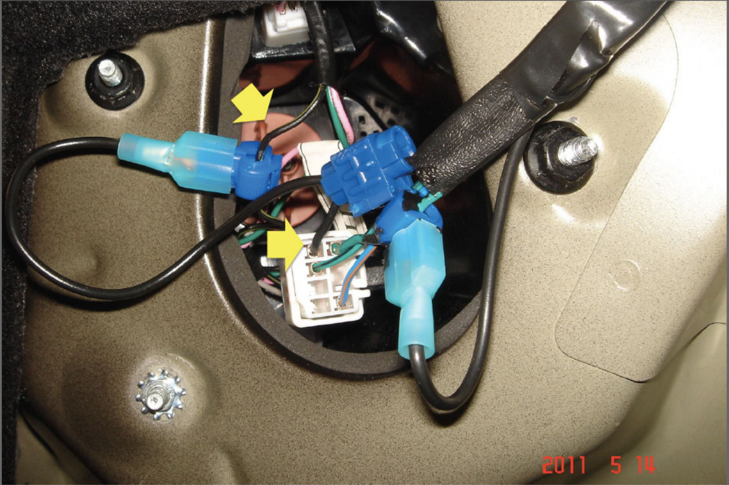
These two wires (Black and Black with strip) need to be connected for quarter panel tails LED to work properly. I used quick splice on one end ,and t-tap on another to make for easier access in future maintenance
