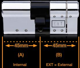
Two measurements are required to determine the size of the cylinder.
