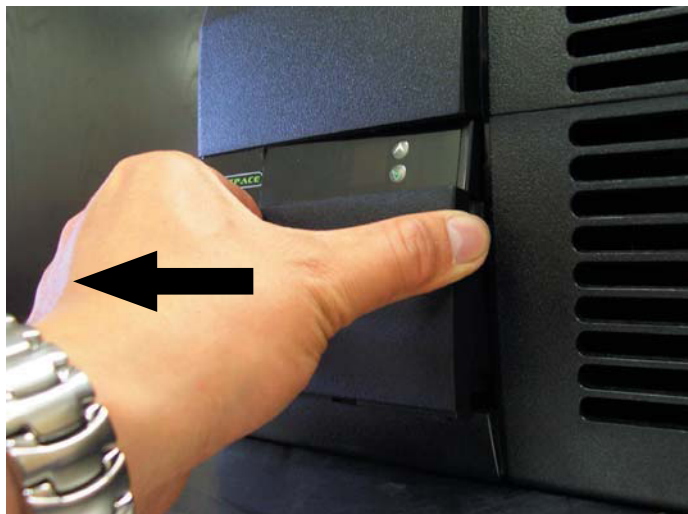
② Angle bottom out and pull out controller.
