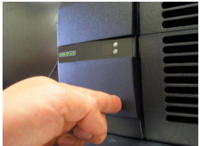
⑫ Push bottom right corner to snap in place.
