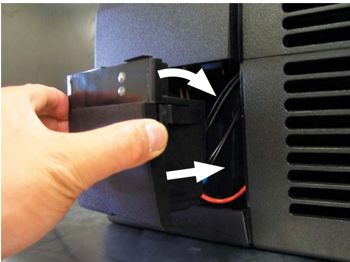
⑪ Slide in controller box by angling top in first.
