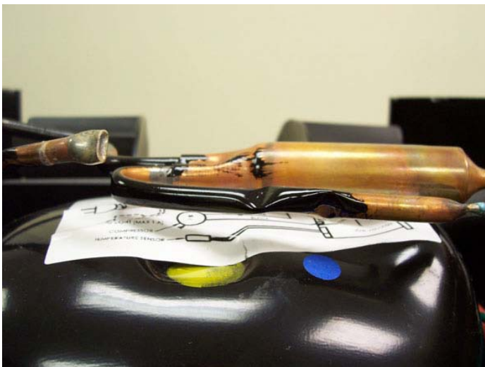
⑤ Above shows copper tubes touching compressor.
