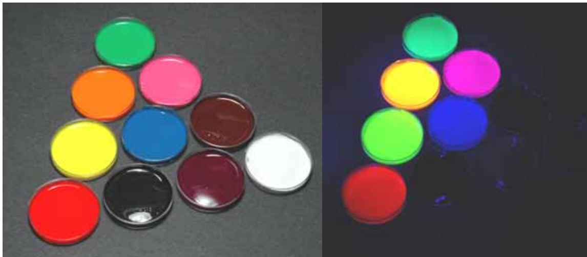
Samples of the ten VIE colors under ambient light (left) and illuminated in a darkened room by the VI light. Note that only the six fluorescent colors show up in the VI light, and that the colors, especially the yellow, appear somewhat different when fluoresced.
