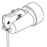
REMORA SHOWN MOUNTED ONTO SOLA LIGHT (O-RING NOT SHOWN)
