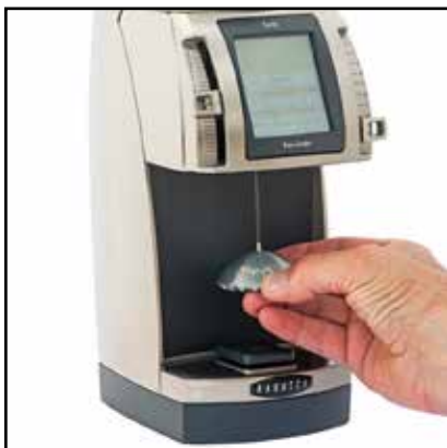
Use the burr calibration tool while the grinder is running.
