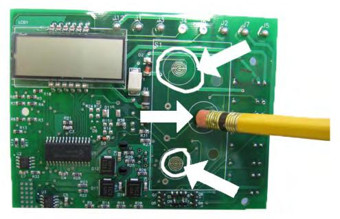
Replace the circuit board in the cover housing. Replace the unit on the base and now you should see the buttons respond like they were new. For extra caution, purchase the STAT rebuild kit to replace the buttons and cover plate.
