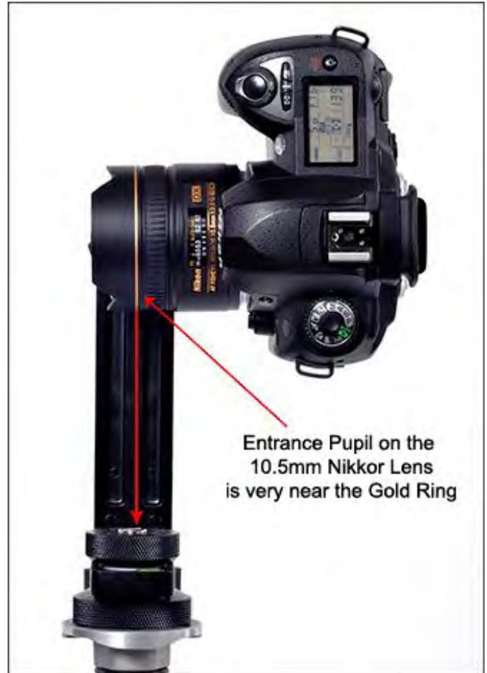
Insert a rail stop as shown and tighten to lock, and remember this position. The upper position is now set, unless you change camera and / or lenses or vary the focal length, it will remain as is.
