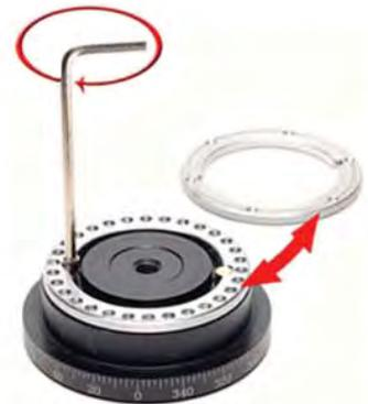
Using the enclosed hex key loosen the inner hex screw enough to release detent ring. Some units may have the hex key tool located inside the tension knob, as shown above left. Place the detent ring with desired side face up. Tighten hex screw and reassemble.
