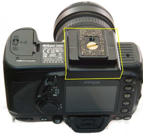
Attach camera plate to camera.
