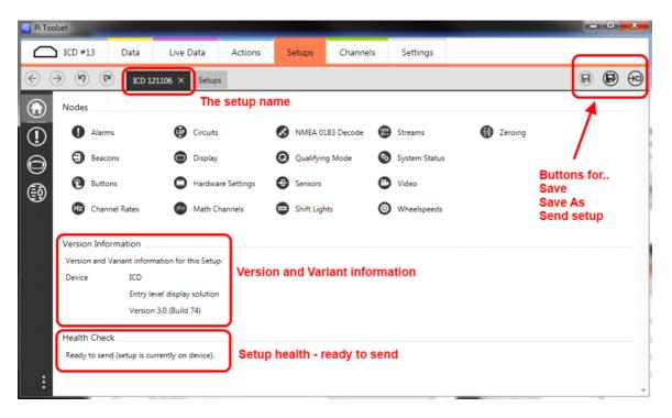
The buttons on the top right side operate that setup. When a change is made to a setup (for example to the logging rates) then Toolset will show that the setup has not been saved with a \* suffix to the setup name;
